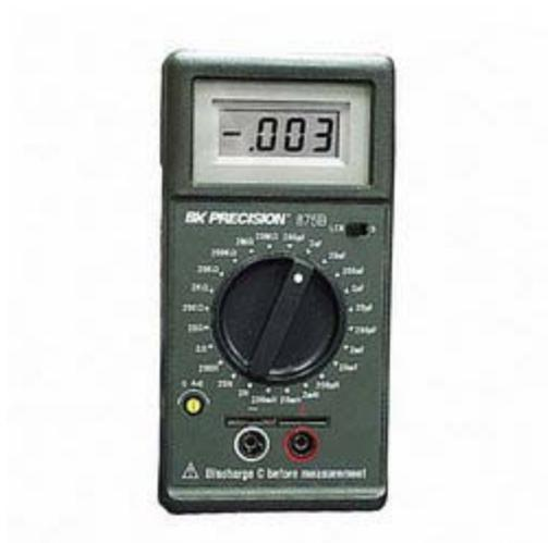
Gambar 3. Alat ukur LCR meter
